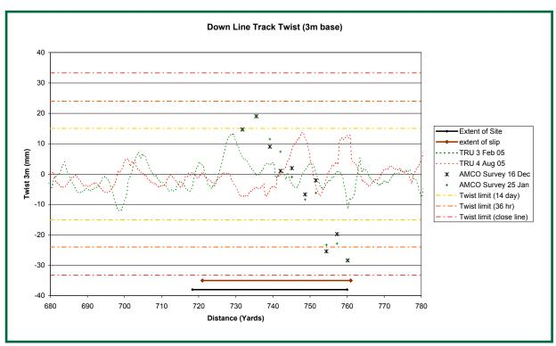
Figure 8: Track twist plotted against distance.
