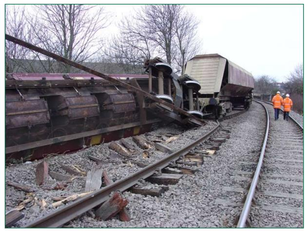
Figure 5: Leading derailed vehicle and track damage.
