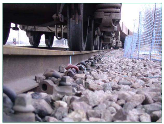
Figure 6: track twist beneath rear part of train.
