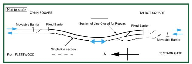
Figure 2: Diagram of lines between Gynn Square and Talbot Square
